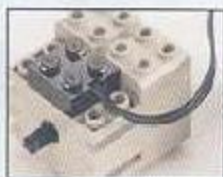
With the wire attached this way, the motor turns one direction.
