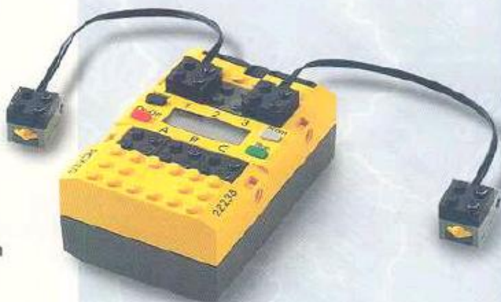
With the wire attached this way, the motor turns one direction.
