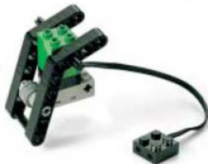
A bumper that uses one touch sensor
