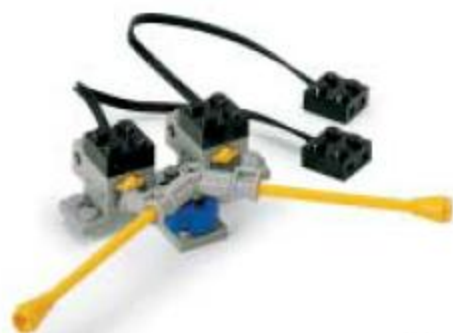
A bumper that uses two touch sensors
